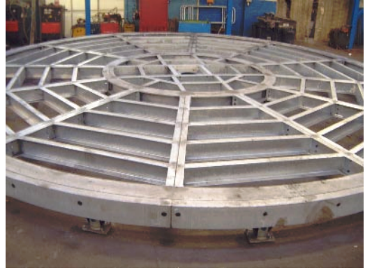
A 9-metre diameter mechanical commercial turntable undergoing construction prior to delivery
