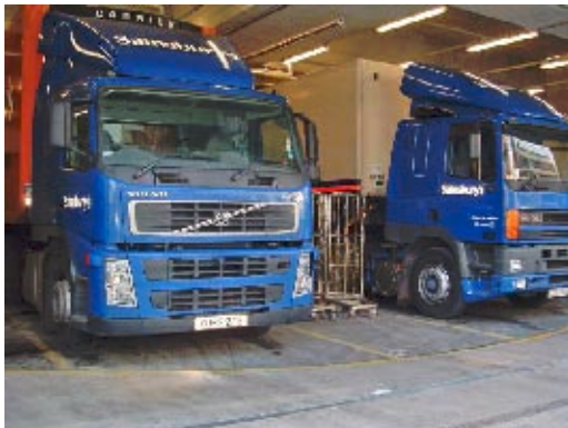
Two fully laden 44 tonne articulated vehicles positioned on board a 17.5 metre, air film turntable.
